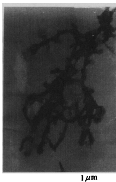
Fig. 6 TEM image of pure PAN particles
